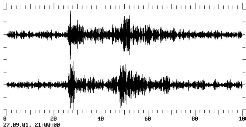
Fig. 8. Correlation seismic traces.
