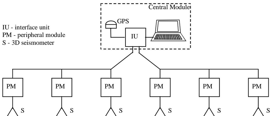
Fig. 5. Block diagram of the *ROSA* system.
