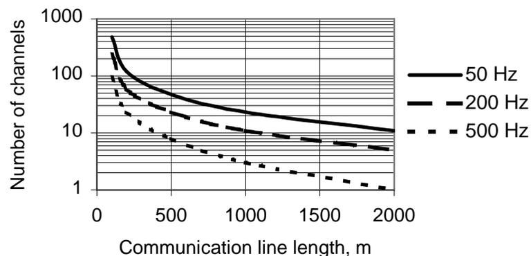
Fig. 6. The maximal number of channels versus the communication line width.
