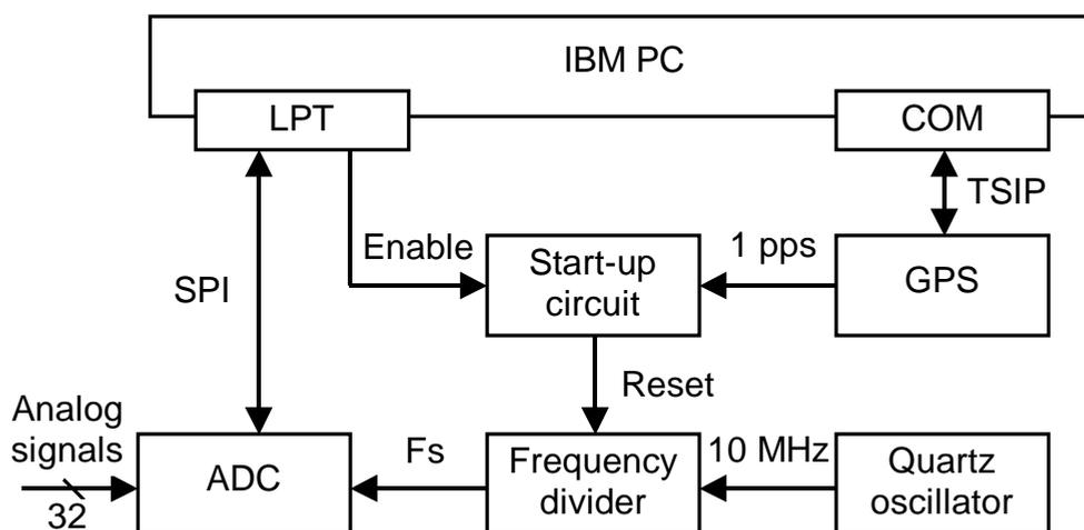
Fig. 2. Block scheme of the measuring block.
